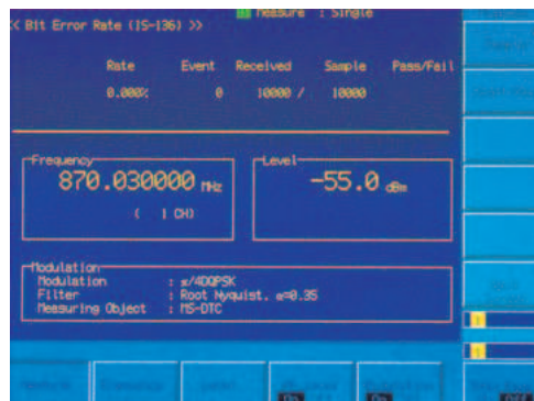
Bit error rate measurement (IS-136A)
