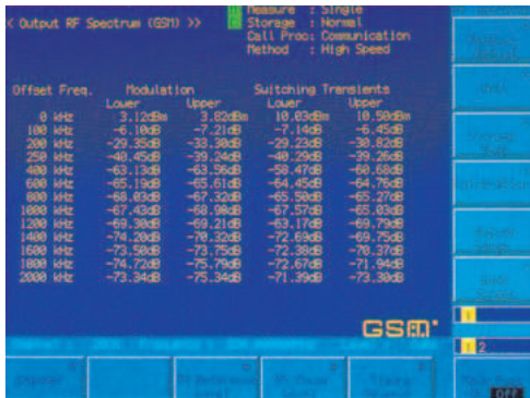
Output RF spectrum measurement (GSM)
